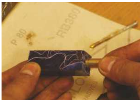
▲ Pic.2 Glue the tubes into the blanks using your preferred adhesive
